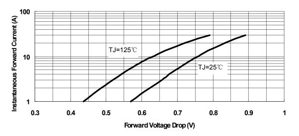
Fig.3-Typical Instantaneous Forward Voltage Characteristics
